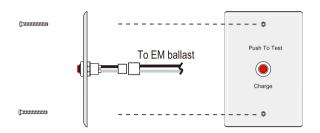
B. Install test switch on fixture surface.
