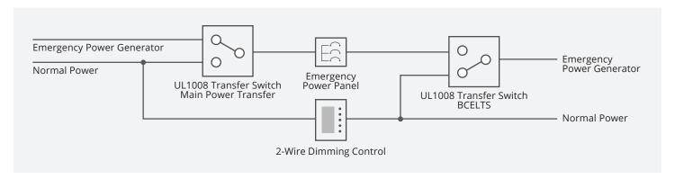
A more common scenario for deploying emergency lighting in the presence of line voltage dimming is to have only a subset of the controlled zone transfer to full on during an emergency. In this situation a UL1008 device must be used in order to facilitate the transfer to emergency power.
