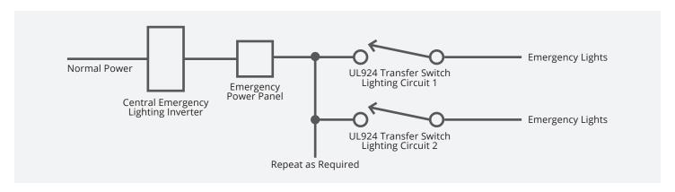
Example 1 is a cost-effective way to achieve code compliance. The arrangement of a single UL1008 device with several UL924 devices means that the UL1008 device performs the transfer of normal power to emergency power while the UL924 devices shunt the loads in the on state. Also note that the emergency lights in this example may also be 0-10V/ DALI dimmed loads when utilized with a UL924 device that incorporates a dimming interface.
