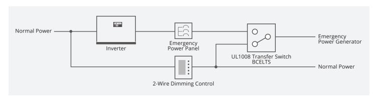
As described in example 3C, an inverter may take the place of a UL1008 device to facilitate the transfer between normal and emergency power. In situations where not all controlled lights are intended to be used for emergency lighting, a UL1008 still must be used to facilitate the transfer into emergency mode. All examples (3A, 3B, 3C, 3D) are fully NEC compliant.
