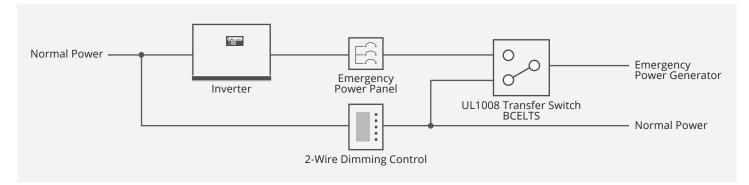
As described in example 3C, an inverter may take the place of a UL1008 device to facilitate the transfer between normal and emergency power. In situations where not all controlled lights are intended to be used for emergency lighting, a UL1008 still must be used to facilitate the transfer into emergency mode. All examples (3A, 3B, 3C, 3D) are fully NEC compliant.
