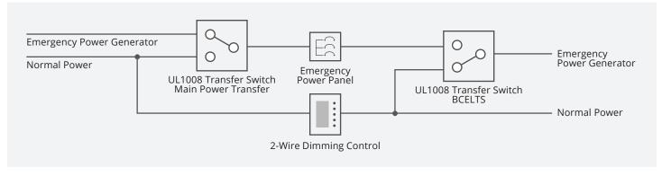
A more common scenario for deploying emergency lighting in the presence of line voltage dimming is to have only a subset of the controlled zone transfer to full on during an emergency. In this situation a UL1008 device must be used in order to facilitate the transfer to emergency power.
