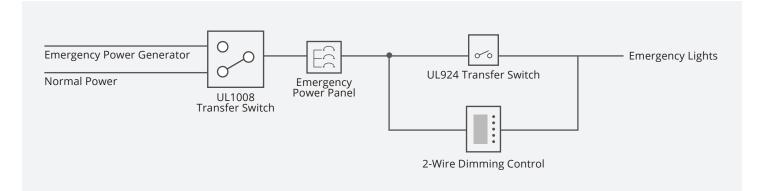
When an upstream 1008 transfer device is utilized to transfer between normal and emergency power, a downstream UL924 device may be used so long as the entire controlled zone is intended to be on during an emergency. If only a subset of the loads in the zone are to fulfill emergency functionality, see example 3B.
