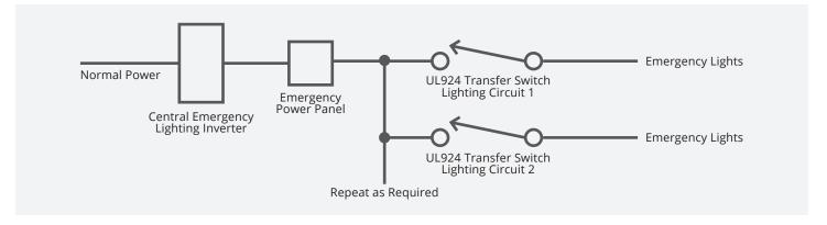
Example 1 is a cost-effective way to achieve code compliance. The arrangement of a single UL1008 device with several UL924 devices means that the UL1008 device performs the transfer of normal power to emergency power while the UL924 devices shunt the loads in the on state. Also note that the emergency lights in this example may also be 0-10V/ DALI dimmed loads when utilized with a UL924 device that incorporates a dimming interface.
