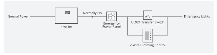
As in example 3A, a UL924 device may be used to facilitate a transfer to emergency levels when utilizing an upstream centralized inverter; no UL1008 device is required in this situation. Do note that the sense wires on the UL924 device must be connected to normal power, not the normally on output from the inverter.
