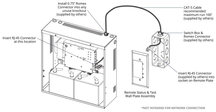
**NOTE:** RJ-45 / CAT-5 Cable is used for direct connection from inverter to remote display only.
