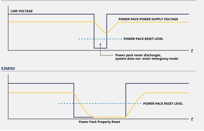
The E3MINI has a field-configurable transfer time, which defaults to a time appropriate for use with smart power packs. Faster (and slower) transfer times are selectable in the field during installation.
