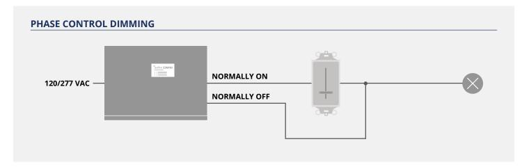
When using a traditional 2-wire dimmer, the dimmed control signal is not sent through the inverter. Instead, the inverter shunts around the phase control dimmer to short circuit the controls in an emergency. Note that while it is possible to operate the lights at a dimmed level in normal operation, when the system goes into emergency mode, the fixtures will be at 100%.
