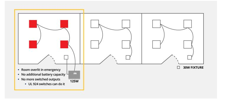
With its multipurpose outputs, the E3MINI smart inverter can divide its power output into three separate zones of emergency lighting, which all operate independently under normal conditions. The rooms are directly connected to and controlled from the inverter, without additional hardware.
