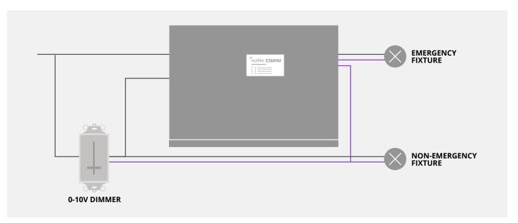
With the switched multipurpose outputs, the E3MINI allows for the integration of 3 zones of 0-10V dimming, each with **independent** control of the output dim level when in emergency mode.
