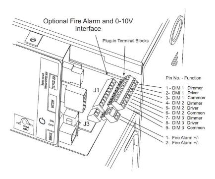
**NOTE** - DALI interface requires the DIM ADJ. to be in the furthest Clockwise (CW) so that the relay opens during Inverter Mode of operation. Dimming requires a DALI signal which the E3MINI Series does not provide.
