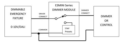
During normal operation, the DIMMABLE EMERGENCY FIXTURE is connected directly to the DIMMER OR CONTROL through the DIMMER MODULE's internal signal relay. Upon loss of power or during a system test, the DIMMER MODULE's internal relay changes state so that the User Presets (5 presets 100% - 20%) will assume control of the dimming level for the DIMMABLE EMERGENCY FIXTURE.
