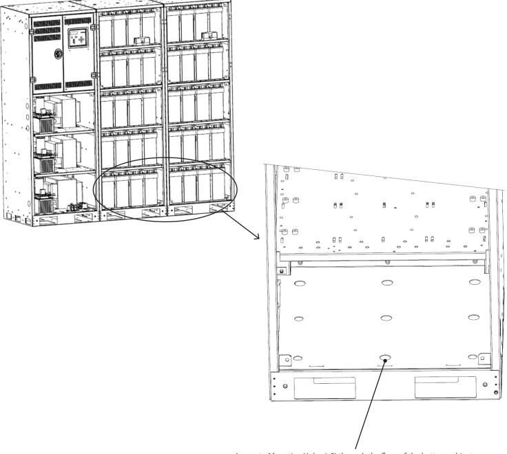
Access to Mounting Holes (x9) through the floor of the battery cabinet. All 9 floor mounts should be installed. Use floor anchoring hardware to secure cabinet. Supplied by contractor.
