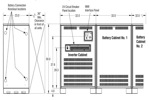
8-12.5KVA Single Phase requires two cabinets (inverter and batteries) 5-12.5KVA Three Phase requires two cabinets (inverter and batteries) 15-18KVA Three Phase requires three cabinets (inverter and batteries)
