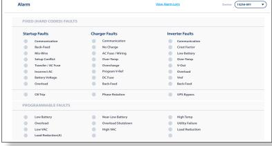
Faults can also be viewed remotely, with email notification available. In conjunction with the remote testing ability, this allows the Isolite inverter tech team to troubleshoot inverter problems remotely.
